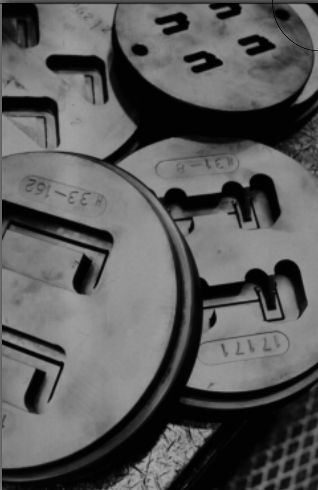
The tools needed for the production of aluminium profiles are manufactured at the Kirkkonummi factory.
